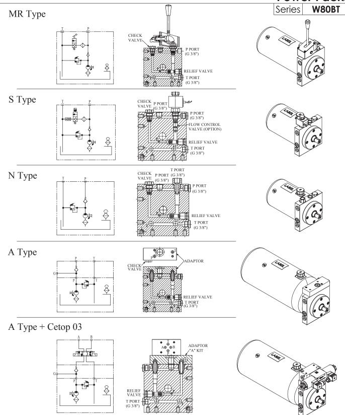
The W80BT power pack series is designed for use with horizontal influence drive system by various engines. These power packs have been designed mostly for agricultural use, but can be used in other fields.
